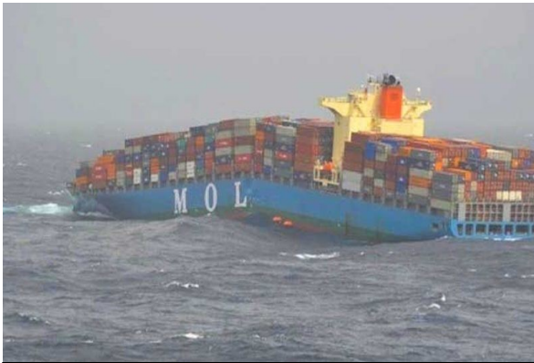
The MV MOL Comfort seen June 17, 2013 breaking in half while underway in the Indian Ocean.
