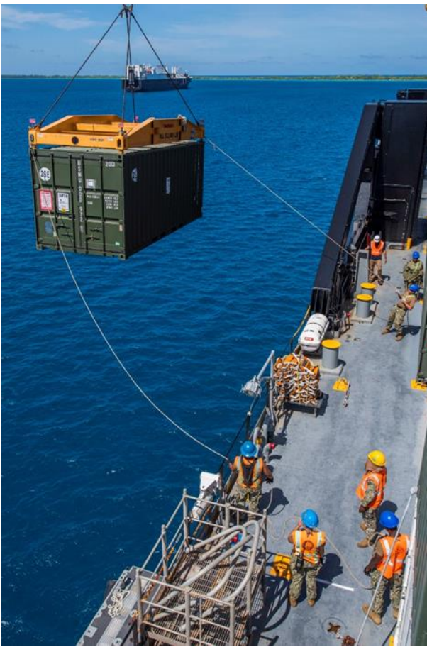
191114-N-CO914-1065 DIEGO GARCIA, British Indian Ocean Territory (November 14, 2019) Sailors keep tension on taglines as a crane lifts a container aboard Military Sealift Command Bob Hope-class roll-on roll-off vehicle cargo ship USNS Seay (T-AKR 302) during an Improved Navy Lighterage System (INLS) training mission. Navy Cargo Handling Battalion (NCHB) 1, NCHB 8, NCHB 11, NCHB 13, Assault Craft Unit (ACU) 1 and Amphibious Construction Battalion (ACB) 1 are participating in the INLS training mission under the direction of Commander, Task Force (CTF) 75 in preparation for upcoming joint cargo handling exercise Native Fury 2020. (U.S. Navy photo by Mass Communication Specialist 1st Class Nathan Carpenter)
