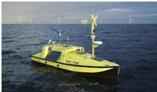
Hugin is the first surface measurement vessel specifically built for the offshore wind sector (Ørsted)
