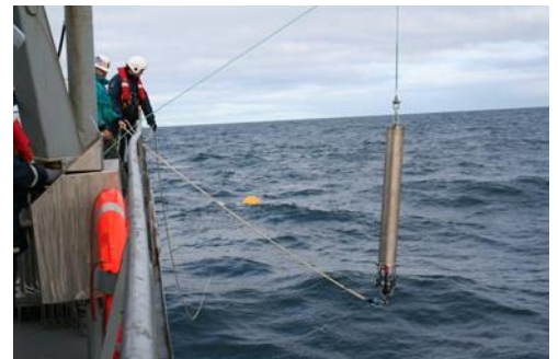
Researchers lowering a hydrophone – a device for recording sound underwater – into the Atlantic Ocean. Dave Mellinger/Oregon State University, CC BY-SA
