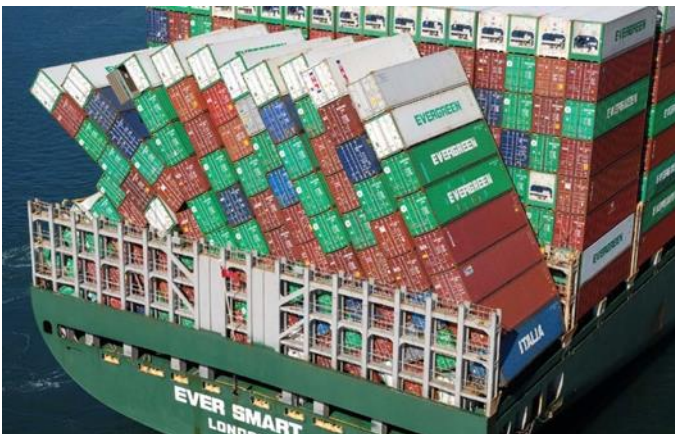
Photo showing collapsed container stacks on the deck of the UK-registered M/V Ever Smart . Photo: MAIB
